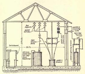
Fig. 139.—Typical transformer sub-station.
